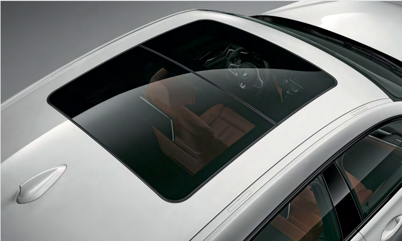
When open, the Panorama glass roof provides a great deal of fresh air. And when closed, it creates a bright, light-flooded atmosphere in the interior. It opens and closes completely automatically at the push of a button, or remotely, and is equipped with slide and lift functions, roller sunblind and wind deflector.
