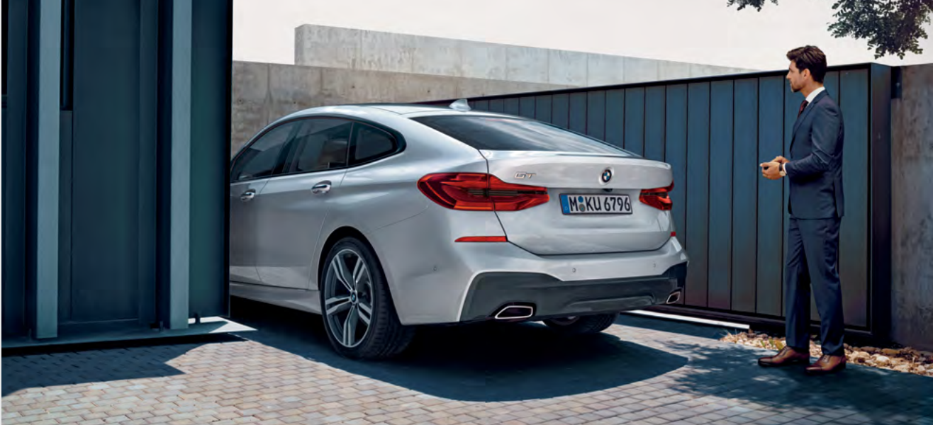
The Remote Control Parking function allows the driver to conveniently get out of the vehicle before parking it via remote control by moving it forward into, or reversing out of a tight parking space or garage. The Remote Control Parking function is activated by the driver once outside the car, with the BMW display key.
