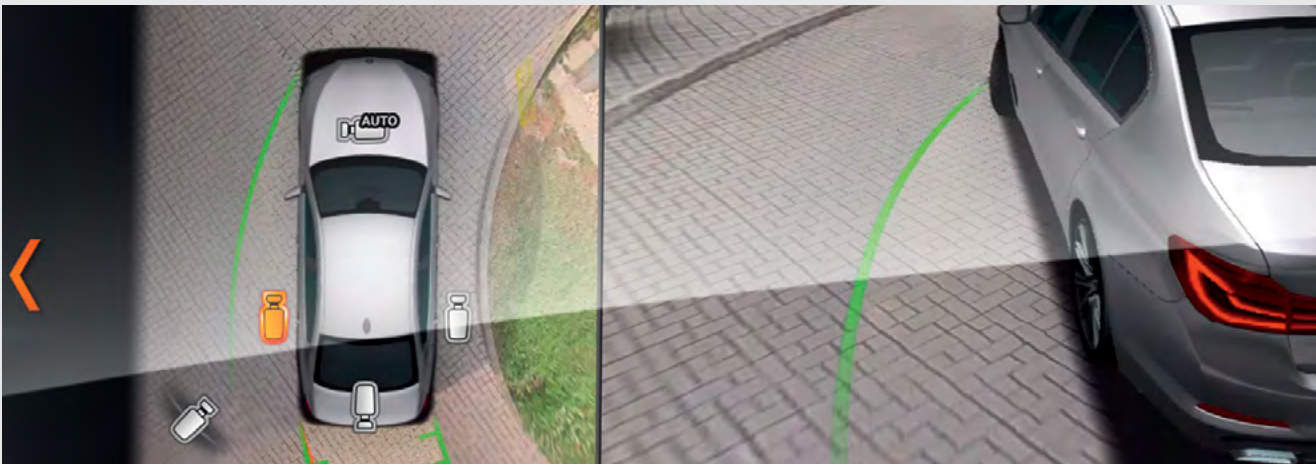
Parking Assistant with Surround View Camera and Reversing Assistant makes parking and manoeuvring the vehicle easier. The Parking Assistant with linear guidance parks the vehicle automatically, parallel or perpendicular to the street. Surround View includes the camera-based functions like Rear View Camera, Panorama View, Top View and 3D View. The cameras in the exterior mirrors as well as at the front and rear of the vehicle allow for a 360° all-around view.
