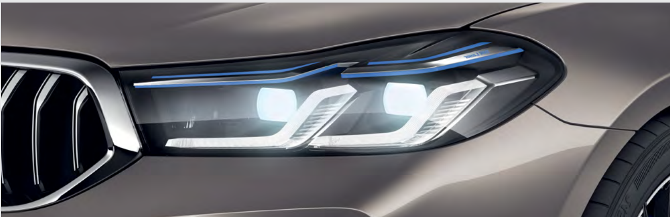
In laser high-beam mode, BMW Laserlight illuminates a range of up to 650 m, nearly twice as far as that of conventional headlights. Better visibility in the dark significantly increases safety. Blue accents and the lettering “BMW Laser” in the headlight also underline the technological standards and the sportiness of the vehicle.
