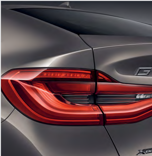
The rear lights with lighting elements in LED technology consist of individual high-performance LED lighting elements and have the characteristic, striking BMW L-shape, meaning that the vehicle is clearly recognisable as a BMW even in the dark.
